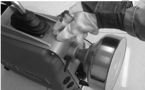
Clutch handle engages cable rotation
