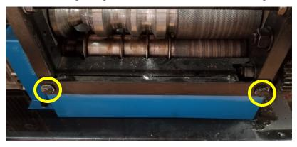
**57.** Install the front guard pieces with 2 bolts as shown and tighten using a 14mm wrench.
