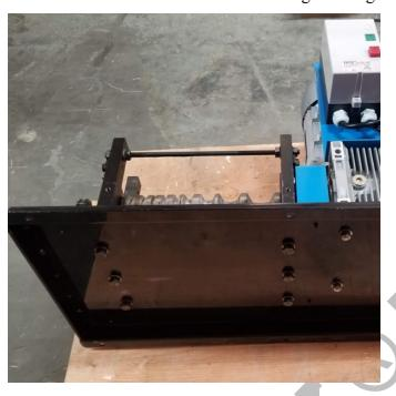
**27.** Use a 17mm wrench to loosen 6 bolts from the bottom side of the roller assembly as shown. **Note:** Do not fully remove the bolts yet.
