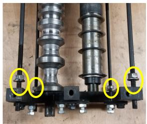
**34.** Use a large puller (pictured is an OTC Brand 6980 brake drum puller) to remove the side plate from the bottom roller assembly. **Important:** Alternate pulling from each shaft to prevent the plate from binding.
