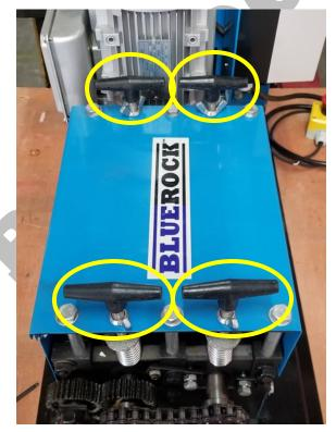
**3.** Remove 4 sets of springs and spring caps from the machine.
