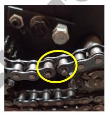
**55.** Install the master link side plate and clip. Use a pliers to fasten the master link clip as shown.
