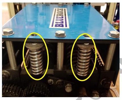
**60.** Screw 4 T-handle blots into the flat brackets as shown until they touch the spring caps. Tighten each bolt an additional quarter inch to set default spring tension.
