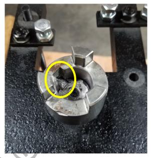
**45.** Place a block of wood across the top of the coupling so it does not get damaged. Squarely tap the block with a hammer until the coupling is fully seated on the shaft.
