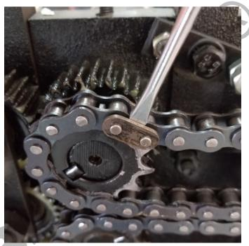
10. Set the chain and master link aside on a clean surface.
