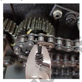
**9.** Use a flathead screwdriver to pry the master link apart as shown.
