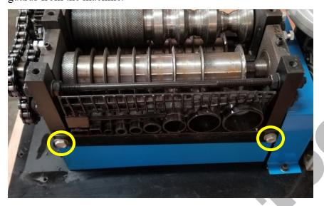
7. Use a 14mm wrench to remove 2 bolts on the rear guard as shown and remove the guards from the machine.
