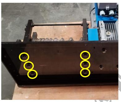
**52.** Very carefully set the upper blade roller into the machine. Then carefully set the upper secondary roller into the machine. **Important:** Be sure the set screws are facing up as shown.
