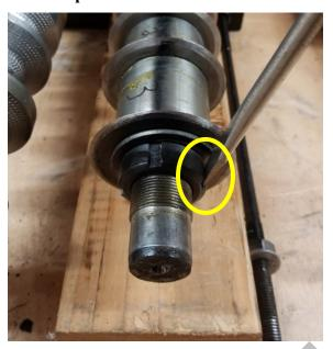
38. Remove spanner nut, washer, blades, and blade spacers from the shaft.
