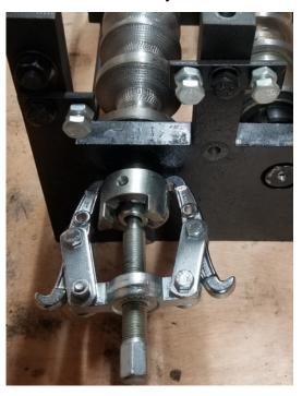
**33.** Use a 14mm wrench to remove 4 nuts and washers from the side of the machine. Then loosen the 4 nuts on the inside of the plate as shown.
