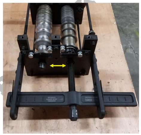
**35.** Pull the bearing from the shaft using a bearing puller as shown.
