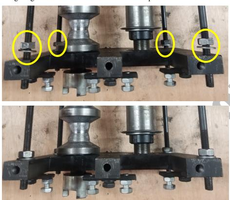
**47.** Place the washers and nuts on the outside of the plate and use a 14mm wrench to tighten.
