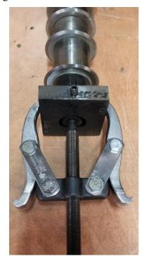
**14.** Use the bearing puller to remove the bearing from the blade shaft.
