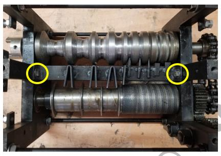
**49.** Carefully prop up the base of the machine with wood blocks so the underside is accessible. Align the holes under the roller assembly with the holes on the base as shown. **Important:** Be sure the motor coupling is aligned and fitted together properly.
