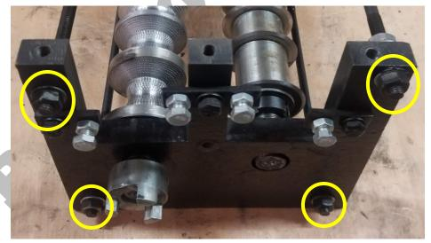
**48.** Install the middle guard and with 2 bolts as shown. Use a 14mm wrench to tighten. **Note:** Turn the roller assembly to be sure the guard does not rub, adjust as needed.
