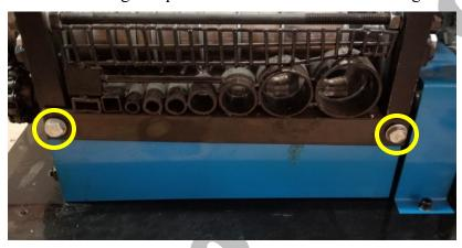
**58.** Set the top cover in place with 2 flat brackets 6 spacer tubes aligned under it. Insert 6 bolts through the holes in the top cover as shown and use a 17mm wrench to tighten.
