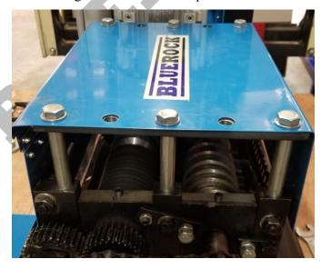
**59.** Set the 4 sets of springs and spring caps in place over the set screws as shown with a small spring inside each large spring.
