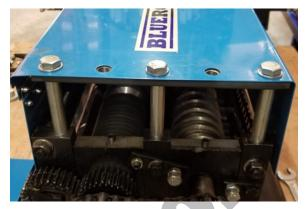
**4.** Use a 17mm wrench to remove the 6 top bolts from the machine.
