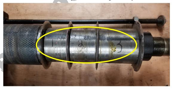
**37.** Place a flat punch against the spanner nut as shown with a wood block supporting the bottom of the roller. Very carefully tap the punch with a hammer until the spanner nut is loose. **Important:** This nut is reverse threaded, loosen by spinning clockwise.
