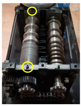
**53.** Use a 14mm wrench to install the upper roller alignment bracket as shown.
