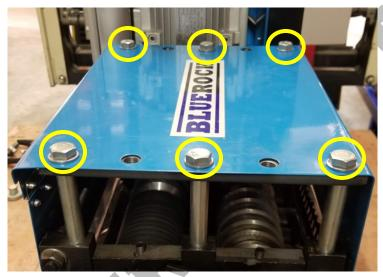
**5.** Carefully lift the top cover away from the machine. Be sure to remove 6 spacer tubes and 2 flat brackets as shown.
