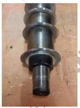
15. Use a marker to number the blade spacers for use during reassembly.
