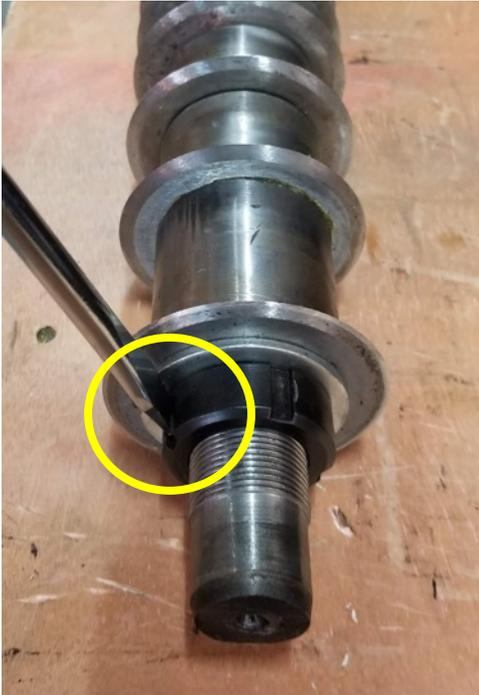
17. **Very carefully** hold the blade assembly and tap the punch with a hammer until the nut is loose. **Note:** This nut is standard thread, loosen by spinning counterclockwise.
