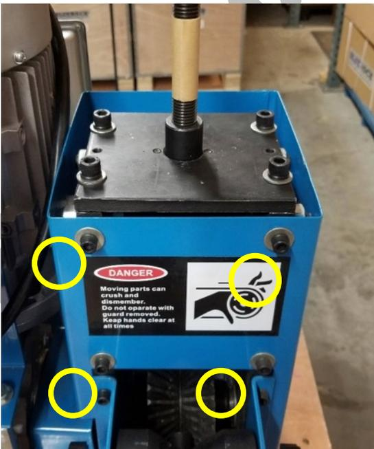
22. Place the top cover over the machine and use a 5mm hex wrench to tighten 2 bolts as shown.
