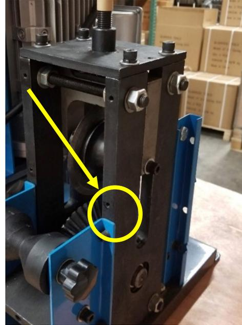
**10. CAUTION: WEAR GLOVES WHEN DEALING WITH SHARP BLADES!** Carefully remove the blade assembly through the opening in the front of the machine. Be extremely careful as the blade may be sharp.
