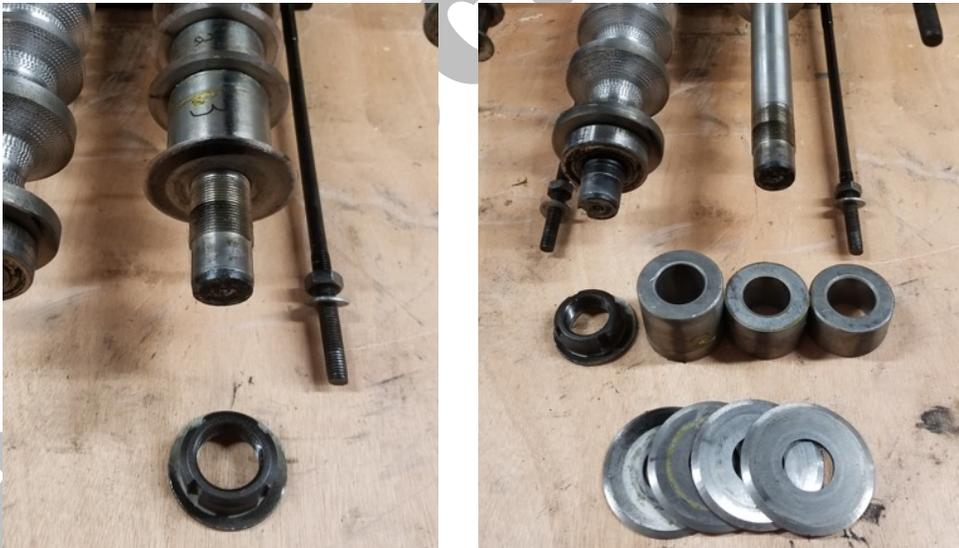
39. Alternate placing new blades and blade spacers on the shaft in the order they came off.
