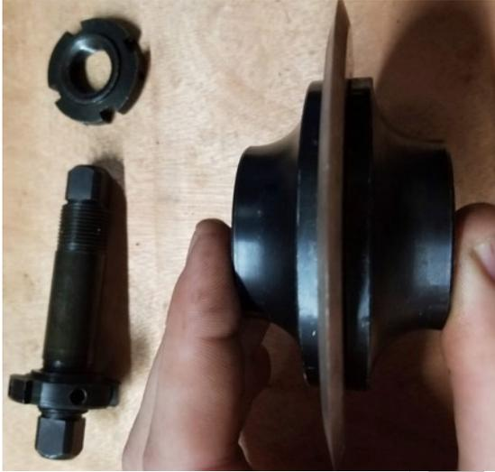
16. Screw the spanner nut onto the shaft until it is flush with the blade carriage. Be sure the flange side of the nut is facing in as shown. **Note:** Do not overtighten the spanner nut or the blade bearings will bind.
