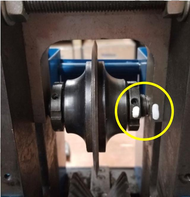
9. Use a 6mm hex wrench to remove the bolts on either side of the blade carriage. **Note:** Carefully hold the blade assembly so it does not fall.
