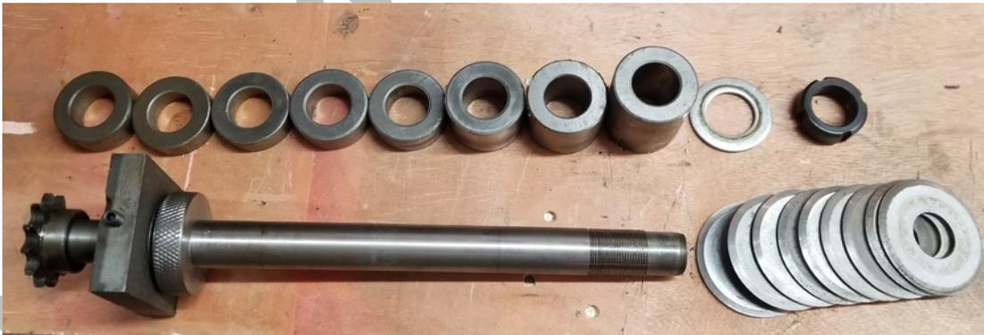
19. Alternate placing new blades and blade spacers on the shaft in the order they came off.
