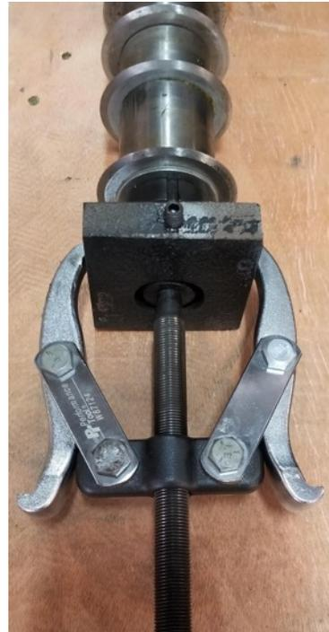
14. Use the bearing puller to remove the bearing from the blade shaft.
