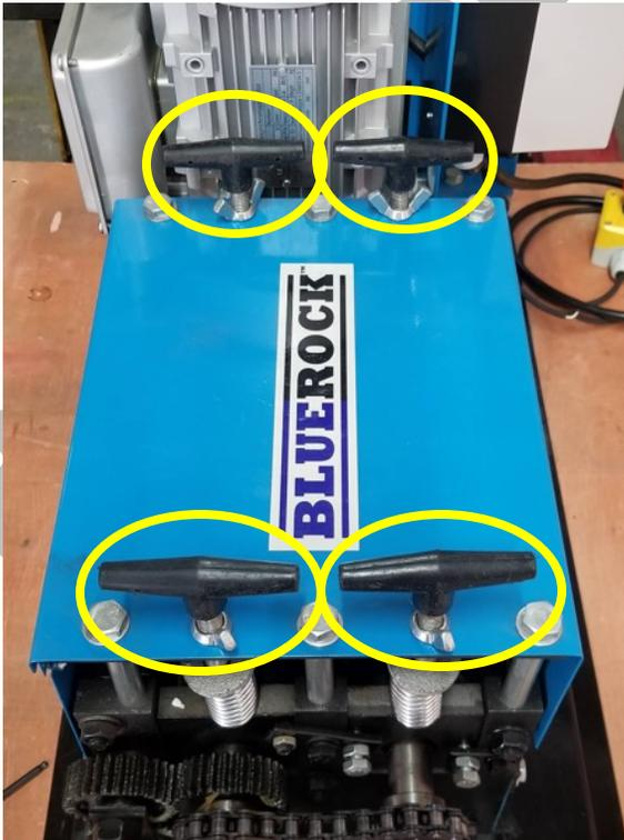
3. Remove 4 sets of springs and spring caps from the machine.
