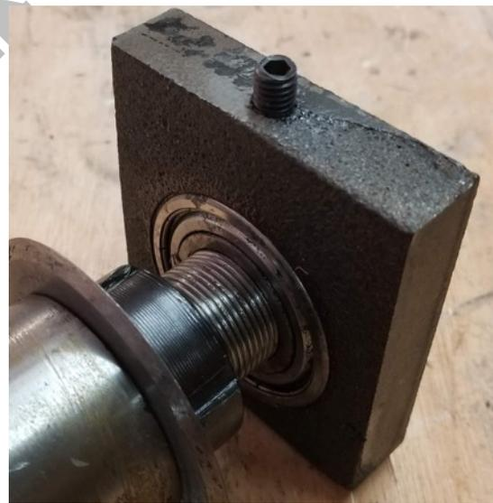
24. Set the blade roller assembly aside until reassembly.
