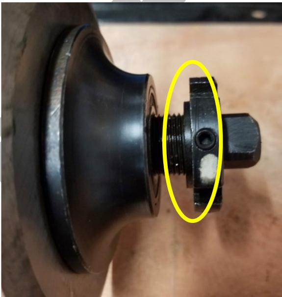
17. Use a 3mm hex wrench to tighten all 4 set screws on the spanner nut.
