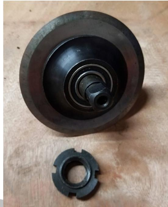
12. Remove the blade carriage from the shaft. Carefully separate the blade carriage and use a 5mm hex wrench to remove 3 bolts holding the blade. **Note:** Do not lose the spacer inside the blade carriage.
