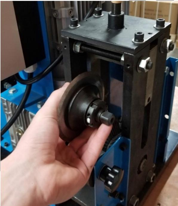
11. Use a 3mm hex wrench to loosen 4 set screws on one of the spanner nuts and carefully remove the spanner nut from the shaft. **Note:** To maintain blade alignment, only loosen one of the spanner nuts.
