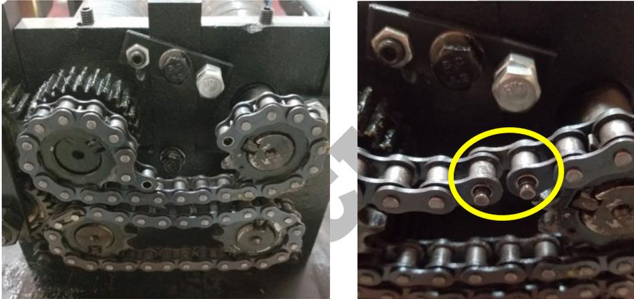
55. Install the master link side plate and clip. Use a pliers to fasten the master link clip as shown.
