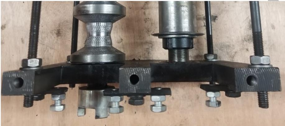
47. Place the washers and nuts on the outside of the plate and use a 14mm wrench to tighten.
