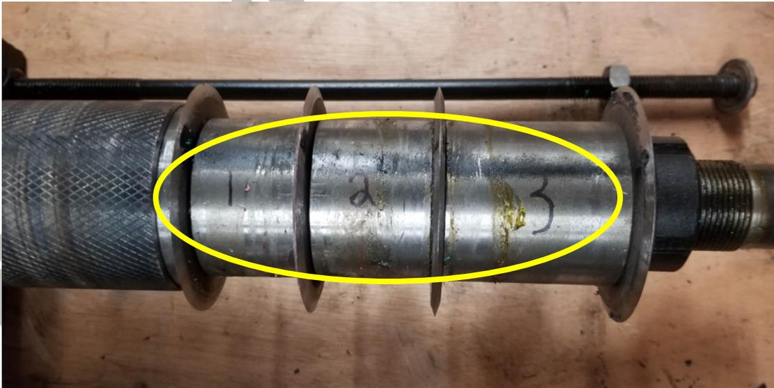
37. Place a flat punch against the spanner nut as shown with a wood block supporting the bottom of the roller. Very carefully tap the punch with a hammer until the spanner nut is loose. **Important:** This nut is reverse threaded, loosen by spinning clockwise.
