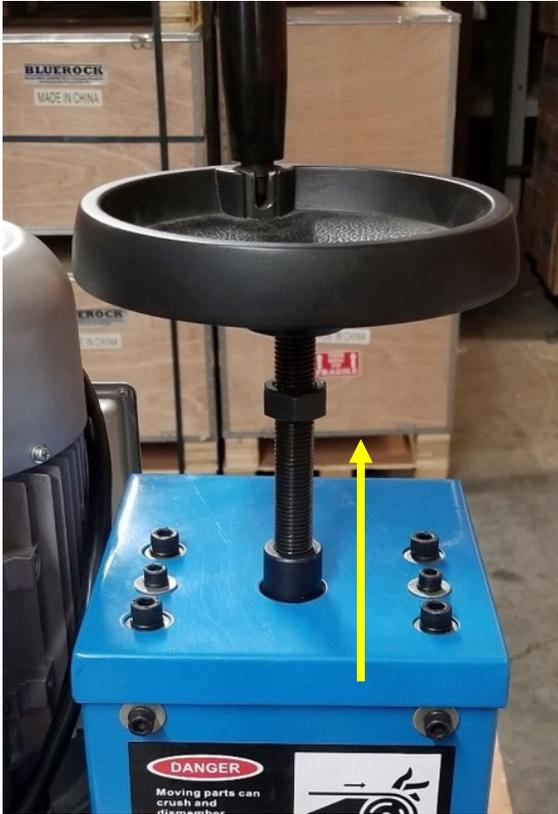
2. Use a 3mm hex wrench to loosen the set screw on the handwheel until it is free from the lead screw.
