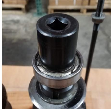
43. Align the side plate of the roller assembly with the lower rollers. Use a rubber mallet to seat the bearings into the housing. Alternate tapping each side as shown to prevent the bearings from binding until the bearings are fully seated in the housing. **Note:** Be sure the nuts on the inside of the plate are loose enough to allow movement.
