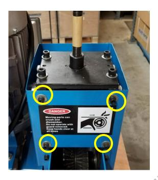
**22.** Place the top cover over the machine and use a 5mm hex wrench to tighten 2 bolts as shown.
