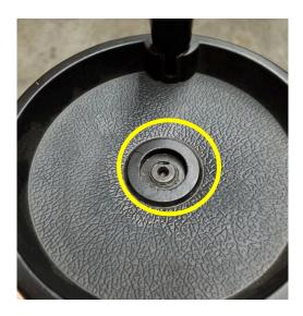
**25.** Use a 3mm hex wrench to tighten the set screw on the handwheel. **Note:** be sure the set screw is aligned with the slot at the top of the lead screw.
