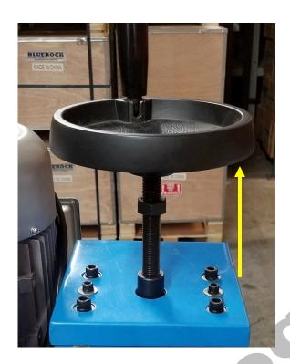
**2.** Use a 3mm hex wrench to loosen the set screw on the handwheel until it is free from the lead screw.
