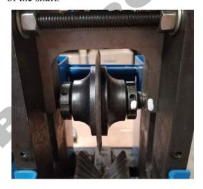
20. Use a 6mm hex wrench to tighten the 2 bolts on either side of the blade carriage
