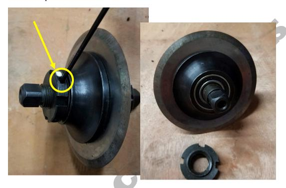
**12.** Remove the blade carriage from the shaft. Carefully separate the blade carriage and use a 5mm hex wrench to remove 3 bolts holding the blade. **Note:** Do not lose the spacer inside the blade carriage.
