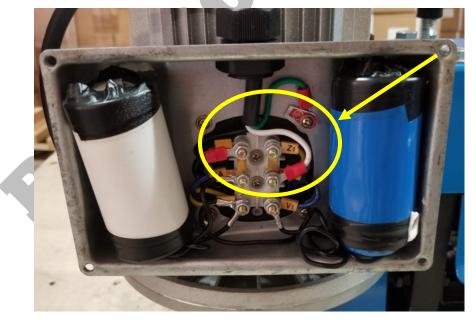
**4.** Use an adjustable wrench to loosen the cord grip located on the top of the capacitor box and pull the power cord out.
