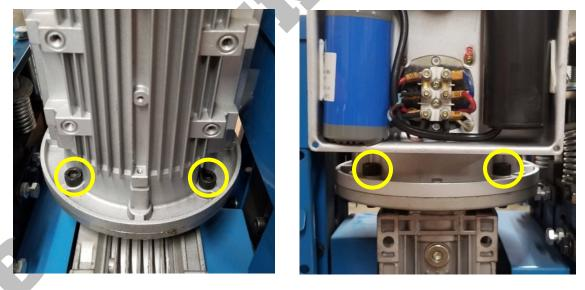
7. Lift the motor away from the machine. **Important:** Be sure to remove the key if it does not come out with the motor.
