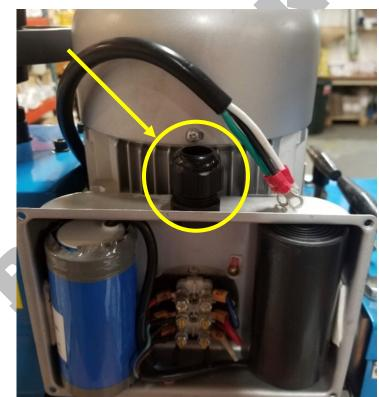
**5.** Use a 14mm wrench to loosen 2 bolts under the motor controller and remove it from the machine. Another 14mm wrench may be needed to hold the nut on the underside.
