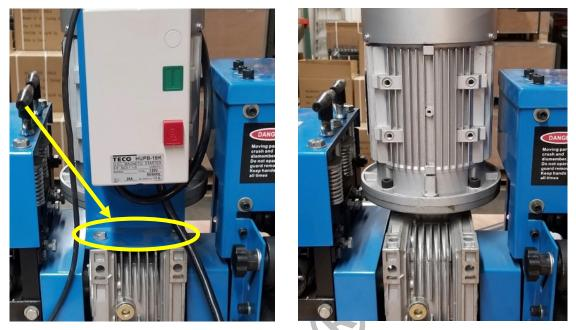
6. Use an 8mm hex wrench to remove 4 bolts from the base of the motor. Note: The nuts may fall from the lower side of the flange when removing the bolts.
