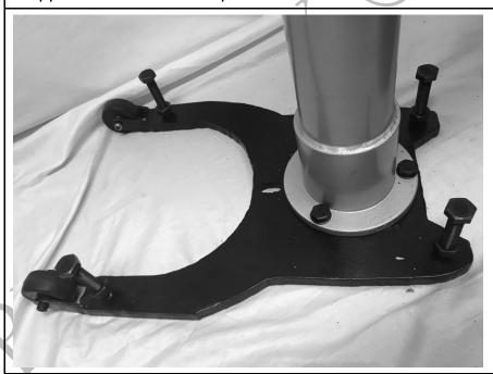
The drill stand has a four-point connection system that connects to the outer stand. This system is the primary system used when setting the drill in the spot and angle needed. CAUTION: Make certain to tighten all set screws and handles on all of these locking components prior to drilling. This is connection system is pictured below:
