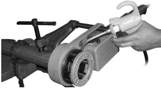
Pipe threading with 11R type die head. We suggest using specific oiler.
