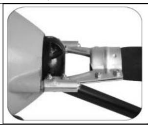
CAUTION: The rubber safety hose must be installed. It protects the user from potential "whipping" action of the end of the sectional cable. Without it installed, damage to persons or property are possible.
